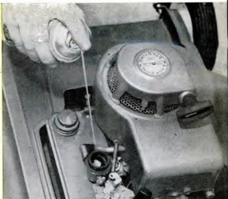
SIMPLE CLEANING of the choke plate and carburetor linkage with solvent often solves hard starting
